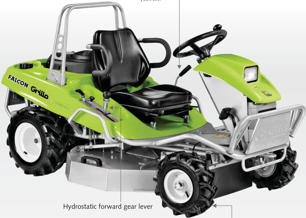
Climber 7.18 has drum brakes on the front wheels which are operated via a pedal to ensure safety on steep slopes and slippery ground.
